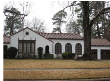
The Spanish Colonial Revival dwelling at 1403 N. 3rd Street has a low-pitched roof and arched casement windows.
